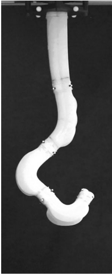
FIG. 21. A spatial cylindrical soft manipulator prototype.
