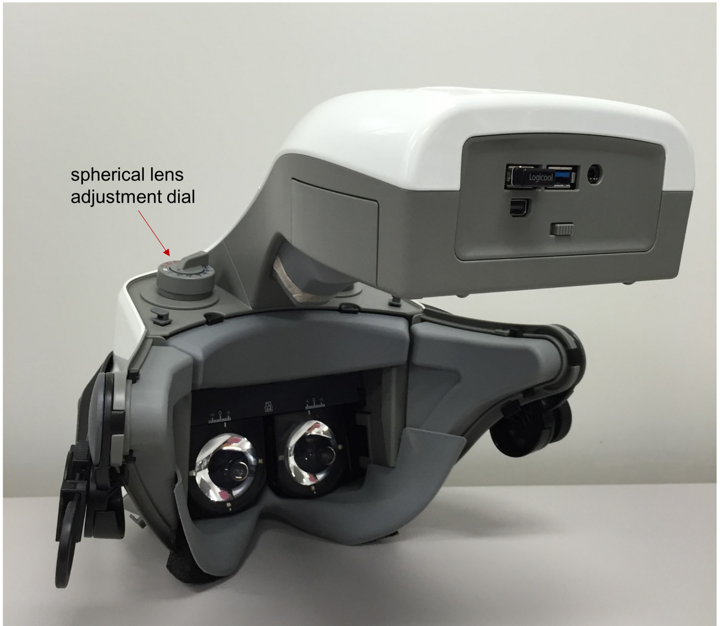
Fig 2. The perimeter unit. The perimeter imo has completely isolated optical systems for the right and left eyes. Stimulus presentation is also independently performed for each eye.
