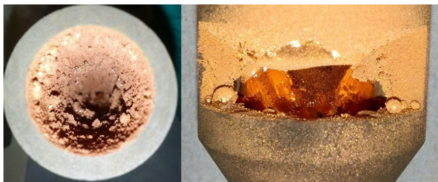
Fig. 6 Image of crucible 6 clogged with copper particles
