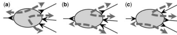
Fig. 1. Walks in bidirected graphs. (a) A valid walk enters and exits a node through opposite edge-orientations. (b) An invalid walk enters and exits a node through identical edge-orientations. (c) Reversing all edge-orientations adjacent to a node results in the same valid and invalid walks
