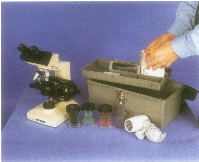
Figure 1 A light weight microscope and a fishing tackle box containing the aspiration and staining equipment including a small hair dryer.
