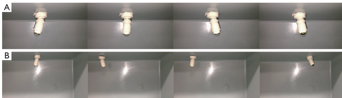
Figure 4 Maneuvering of the wireless steerable endoscope system while suspended on an imitation chest wall: (A) adjustment of viewing direction in situ ; (B) reposition by sliding movement.
