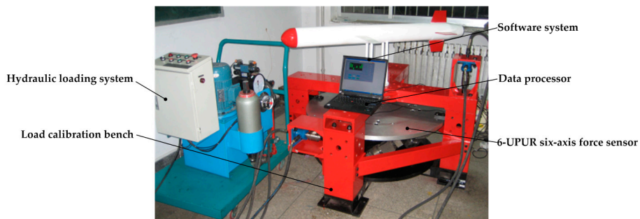
Figure 12. Diagram of the calibration experiment system.
