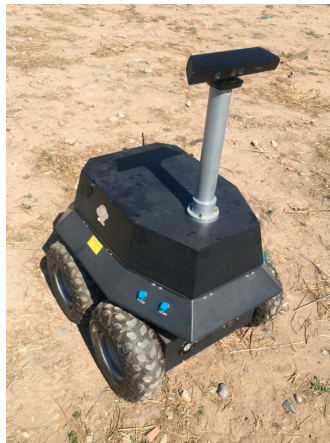
Figure 5. The RGB-D camera mounted on the moving platform.
