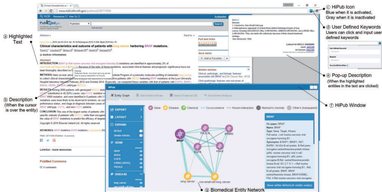
Fig. 1. Overview of the HiPub application. (a) HiPub annotates and highlights biomedical entities in texts. (b) HiPub will display basic information of a highlighted entity when the cursor moves over it. (c) HiPub icon for turning on/off this application in the Chrome browser. (d) Users can click the icon to highlight and add user-defined entities to the biomedical entity network. (e) HiPub will display detailed information of a highlighted entity in a pop-up window when the entity is clicked. (f) HiPub window visualizes recognized entities in texts as a network, allows users to add entities from similar articles, provides search query links for external databases, and performs enrichment analysis for GO terms/KEGG pathways. (g) The biomedical entity network visualizes the relations between entities in a text. The network integrates context-specific entity-relationships extracted from the text and known relationships from external databases for discovering knowledge. Light blue and grey edges represent context-specific and known entity-relationships, respectively. Width of light blue edges represents the frequency of co-occurrence between two entities in the text. The darker grey edge represents the number of evidences supported by external sources
