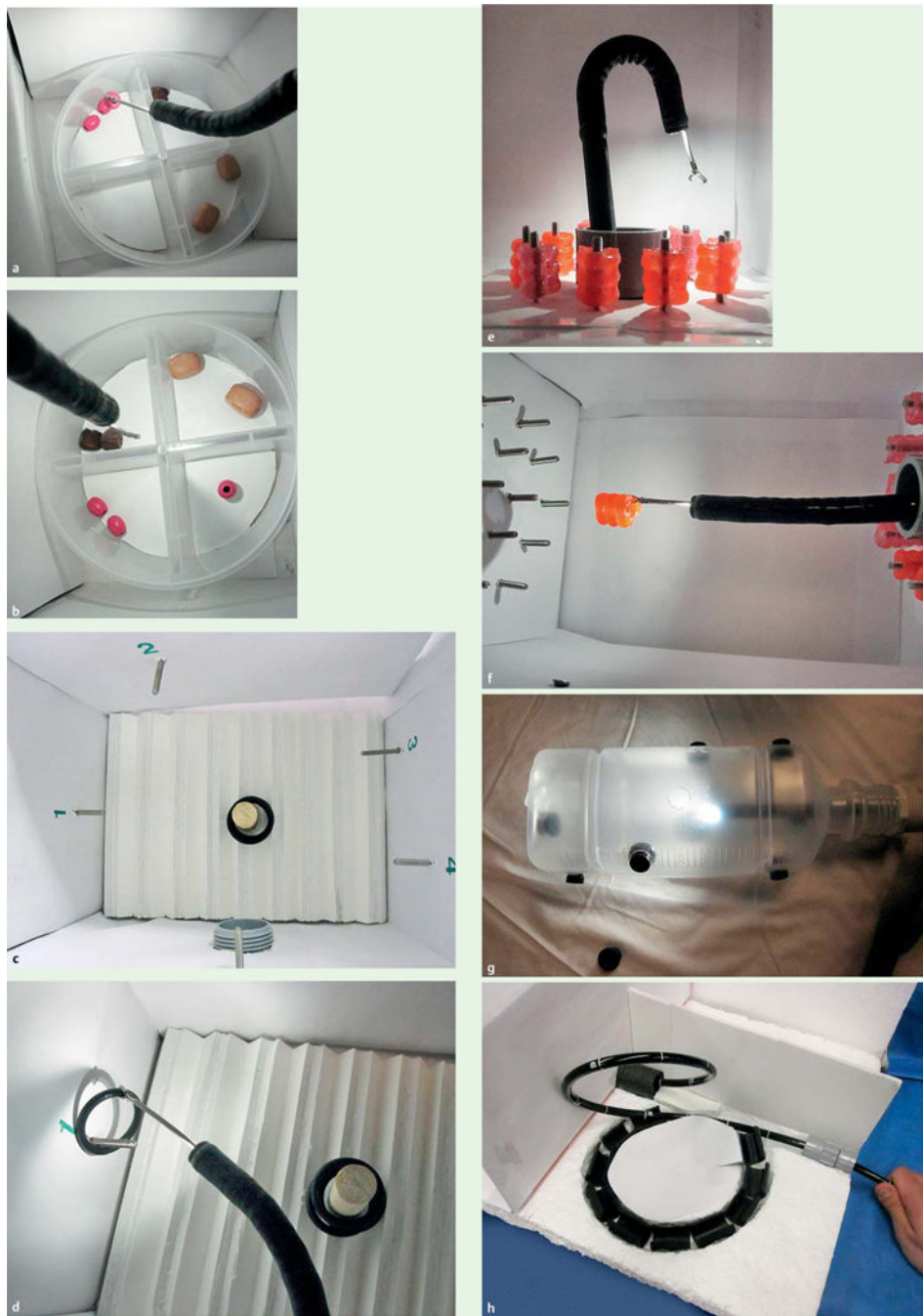
Fig.2. Endoscopic part-task training box alpha prototype. a,b Knob control, with use of forceps to move objects between compartments. c,d Torque, with use of forceps to pick up rings from the center post and place on pegs. e,f Retroflexion, with use of forceps to pick up objects in retroflexed position and place on forward wall. g Polypectomy, using snare to grasp polyps. h Loop reduction, which simulates loop formation and allows a realistic loop reduction maneuver.
