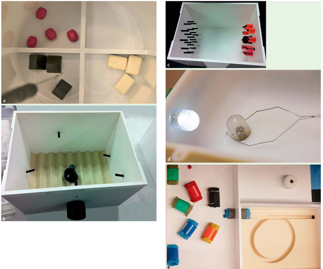
Fig.3. Endoscopic part-task training box beta prototype. a Knob control. b Torque. c Retroflexion. d Polypectomy. e Loop reduction and navigation.
