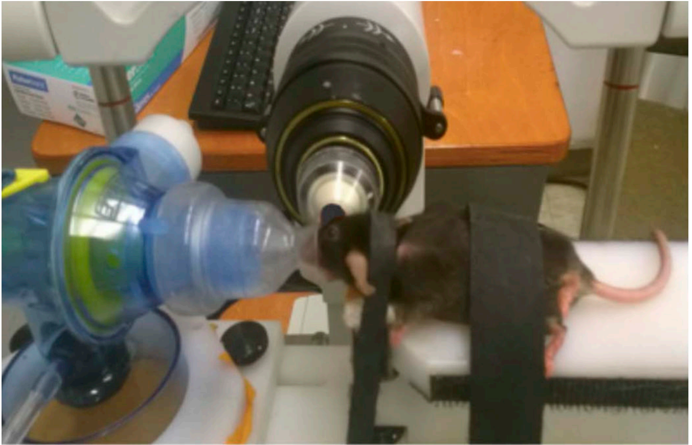
Figure 5. Placement of a mouse on the custom designed platform for corneal imaging. The anesthesia delivery system is visible to the left of the image and the objective of the corneal confocal microscope with tomocap installed is at the center of the image.
