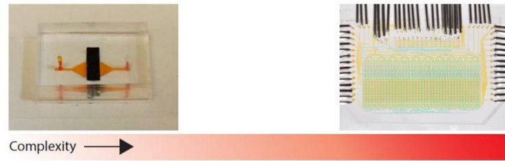
Figure 5. Complexity of Microfluidic Chip Design Depends on Desired Experimental Output Simple microfluidic designs (left) do not equate to less information in comparison to complicated designs (right). Rather, the complication level of each design depends on the required information from the experiment whether it be spatio-temporal dynamics of wound response (left) or cellular response to dynamic, temporal inputs (right, image courtesy of Savas Tay at the Institute for Molecular Engineering at the University of Chicago).
