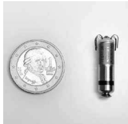
Figure 3. Micra Transcatheter Pacing System. Reproduced with permission of Medtronic.
