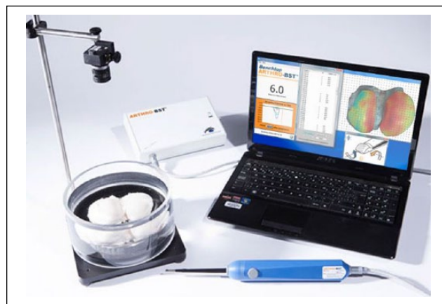
Figure 2. Benchtop version of the Arthro-BST with the testing chamber and the camera-positioning software. The laptop screen shows streaming potential (electrical potential in mV) measured by each of the 37 microelectrodes during indentation and the display of the corresponding Arthro-BST QP (A.U.).
