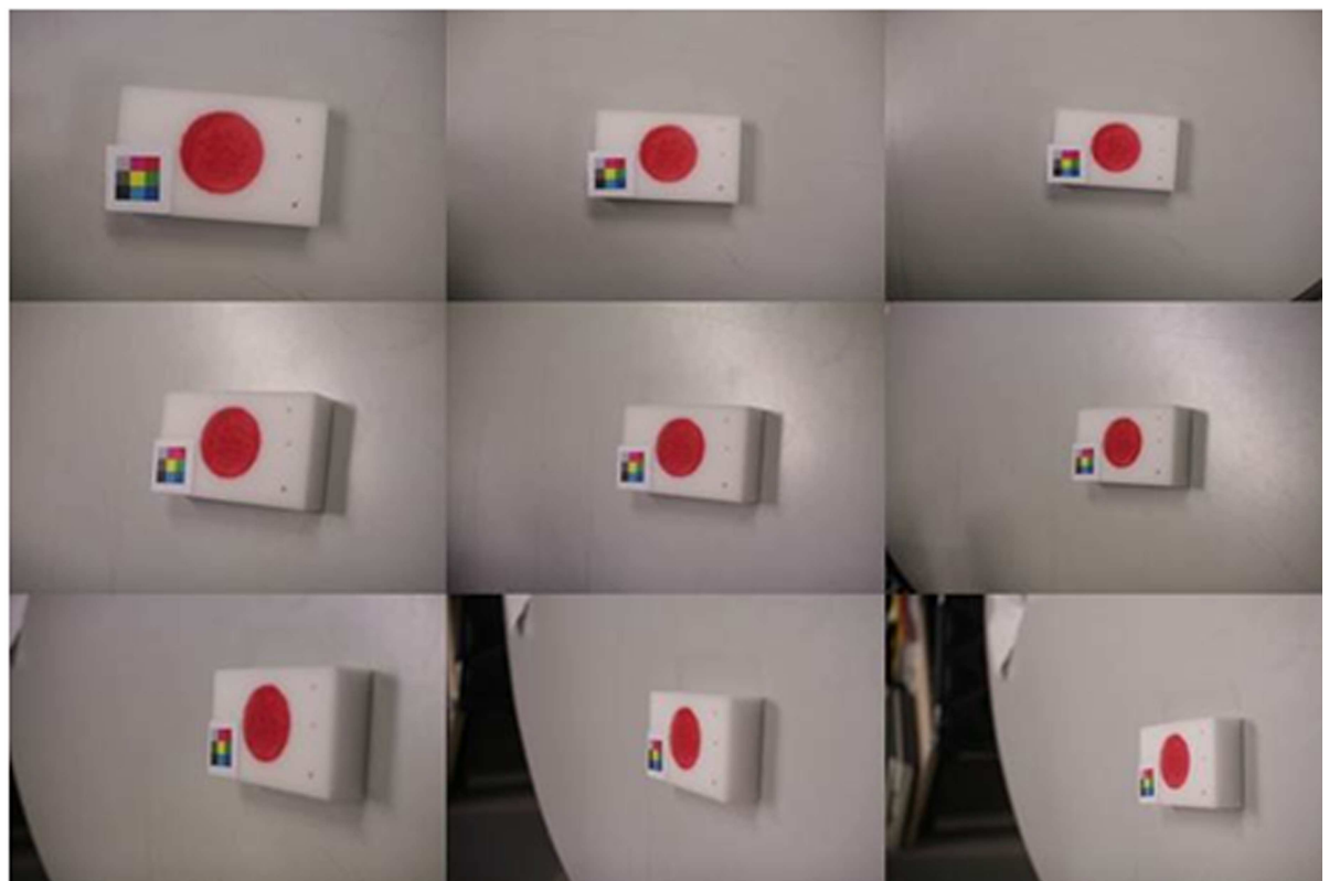
Fig 3. Experimental model for calculating the error rate of color patch method. (A) The capturing system (B) Images captured from 30, 40, and 50 cm distances and at 30, 60, and 90 angles.
