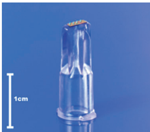
FIG. 2. The experimental MicronJet needle device.
