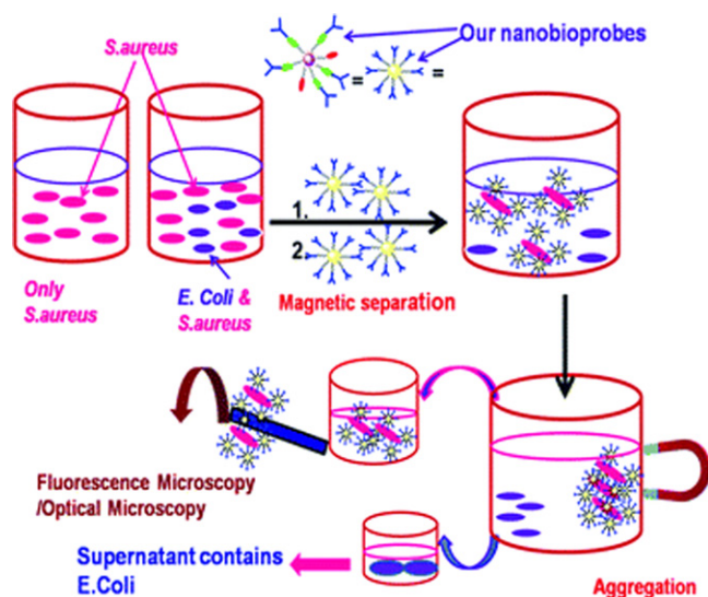
Figure 14. Schematic demonstration of pathogen detection by antibody-modified-fluorescent-MPA-Au-Fe 3 O 4 nanocomposites. (Reprinted with permission from D Bhattacharya et al 2011 J. Mater. Chem. 21 17273. Copyright 2011 Royal Society of Chemistry.)
