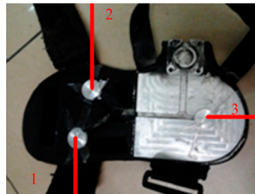
Figure 3. The placement of GRF sensors in the wearable shoe. Two GRF sensors are arranged on the forefoot and one sensor is placed on the heel. The labels 1, 2 and 3 represent the three sensors.
