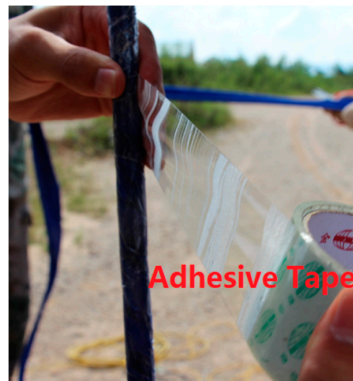
Figure 5. Protective adhesive tape layer.
