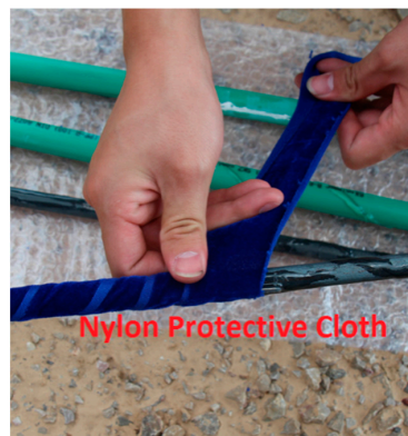
Figure 4. Protective nylon cloth layer.
