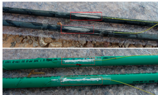
Figure 3. Protective epoxy resin layer for bare fiber.
