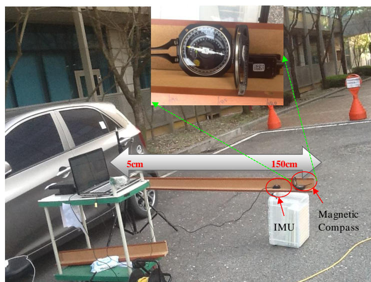
Figure 21. Moving IMU in an exact straight line, by sliding the sensor on a straight wooden support. In close-up is shown a very precise magnetic compass for reference heading.
