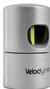
Figure 2. Velodyne 32E LiDAR sensor, employed in this study.
