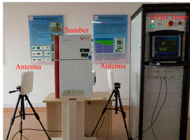
Figure 14. Wireless measurement environment.
