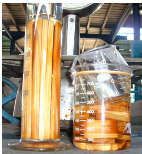
Figure 1. Styrene impregnation of the samples.
