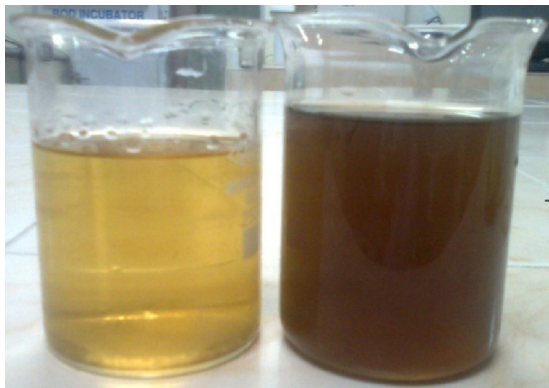
Fig. 2. change of color from yellow to brown indicating the formation of silver nanoparticle.
