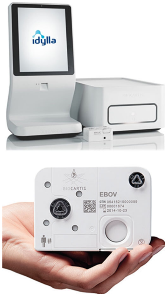
Figure 1. The Idylla™ molecular diagnostic platform. The console is a touch-screen-operated computer supplemented with barcode scanning and communication capabilities and works as a local command center where sample information is entered, tests are initiated, and test results are displayed. The instrument executes a test-specific protocol within the cartridge through multipurpose instrument-cartridge interfaces. Each instrument has a computer, memory and a variety of sensors on board. A single instrument measures 30.5 × 50.6 × 19 cm and weighs 20 kg. Up to 8 instruments can be connected to a single console to accommodate higher-throughput needs. The total power consumption of an installation consisting of a console and an instrument is as low as 200 W. The cartridge is a single-use, disposable plastic consumable with all necessary reagents and controls onboard in lyophilized or liquid form. After the clinical sample is loaded into the cartridge, the latter is closed with an airtight seal and placed in the instrument, which then automatically executes a predefined assay protocol, including the complete measurement and analysis of the data. The cartridge contains an extraction component and a polymerase chain reaction (PCR) disk with 5 individual chambers in which the reverse-transcription PCR takes place. In each chamber, up to 6 differently fluorescent–labeled reporter dyes can be detected. Cartridges do not require cold chain transport and are stored at ambient conditions. This figure is available in black and white in print and in color online.
