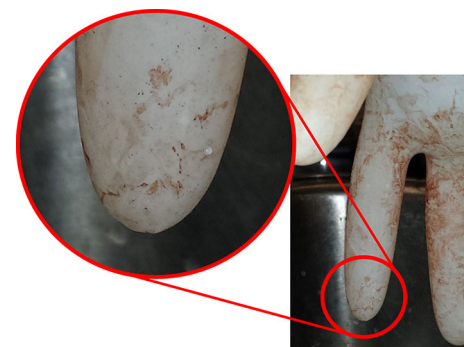
Fig. 2 A microperforation detected as a water droplet during ASTM standard testing is shown.
