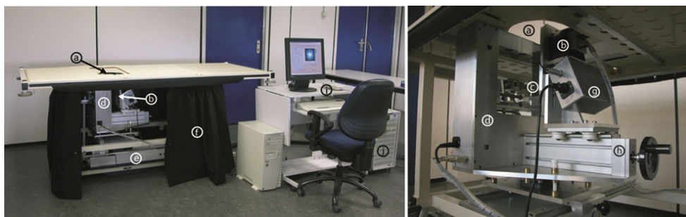
Fig. 1 The Twente Photoacoustic Mammoscope. (a) Aperture for breast insertion. (b) Ultrasound detector matrix. (c) Glass window. (d) Scanning system compartment. (e) Q-switched Nd-YAG laser operated at 1,064 nm with 10-ns pulses. (f) Laser safety curtain which is drawn around the instrument during the measurements. (g) Interface electronics between
