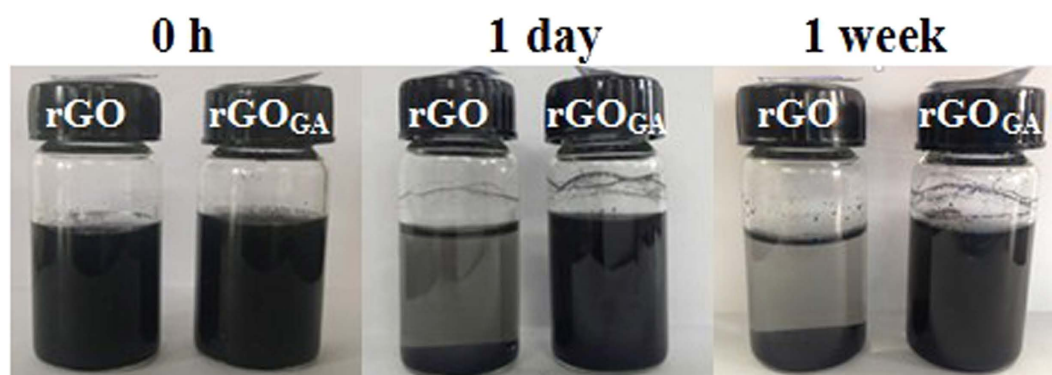
Figure 2. Dispersions of rGO and rGO GA in aqueous solution at different time intervals (~1 mg/mL).
