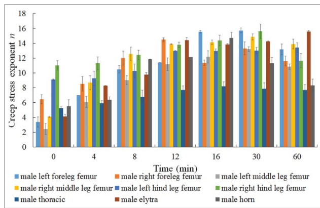
Figure 5. Creep stress exponent of different parts of a male dung beetle.
