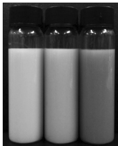
Fig. 2. Curcumin-loaded nanoemulsions prepared with various emulsifiers under high-pressure homogenization conditions of 15,000 psi and 4 cycles. (left: Tween-20 only, middle: Tween-20+SM, and right: Tween-20+SL). Tween-20, polyoxyethylene (20) sorbitan monolaurate; SM, sorbitan monooleate; SL, soy lecithin.
