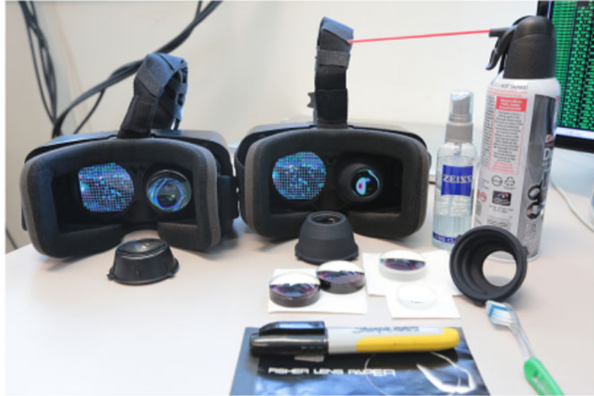
Fig. 1. Photograph of VMD molecular scene on Oculus DK2 HMDs with stock oculars (left) and new high quality oculars with self-assembled optics (right). The HMDs are shown with left ocular removed, allowing the OLED display panel to be seen, showing the OSP stereo perspective reprojection with the HMD lens geometric distortion correction mesh superimposed.
