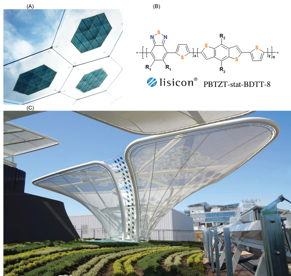
Figure 1. Images of A) a commercial module fabricated by BELECTRIC OPV, B) chemical structure of the polymer PBTZT-stat-BDTT, and C) large scale deployment of BELECTRIC OPV modules at the Universal Exhibition Milan 2015. [7,8]
