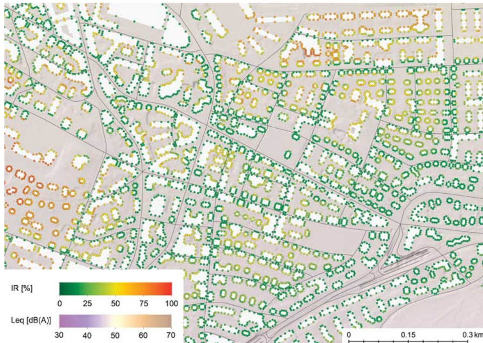
Figure 8. Aircraft noise map showing both L_{eq} and IR during daytime (16 h). Intermittency ratio ( IR ) has been calculated for individual facade points on the map, marked as small dots. The map section shows an area north of the city of Zurich in vicinity of Zurich airport.
