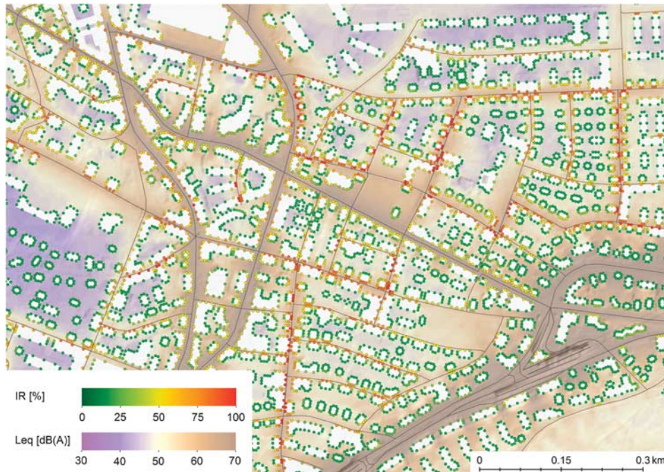
Figure 7. Road traffic noise map showing both L_{eq} and IR during daytime (16 h). Intermittency ratio ( IR ) has been calculated for individual facade points on the map, marked as small dots. The map section shows an area north of the city of Zurich in vicinity of Zurich airport.
