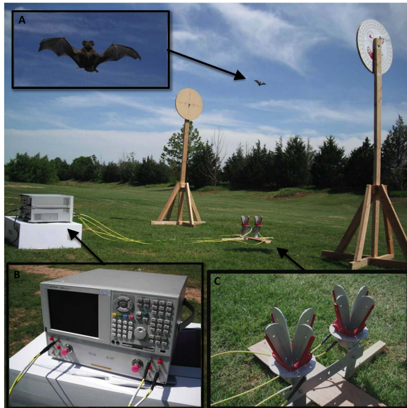
Figure 2. Laboratory equipment setup for controlled measurements. (A) Suspended Brazilian free-tailed bat specimen. (B) Agilent E8364B network analyzer with dual transmit and dual receive channels. (C) Quad-ridged dual-polarization antennas.
