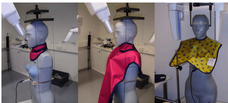
Figure 2 Lead shield for thyroid only (Shield 1, left); lead shield for thyroid, breasts and abdominopelvic region (Shield 2, middle); and lead apron for breasts and upper abdomen (Shield 3, right).
