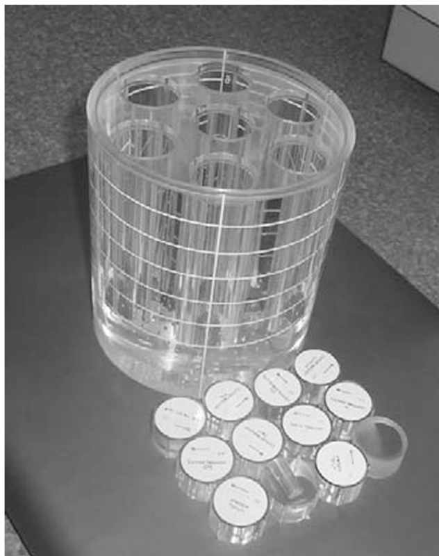
Figure 1 SEDENTEXCT (safety and efficacy of a new and emerging dental X-ray modality) IQ (image quality) phantom housing and inserts.
