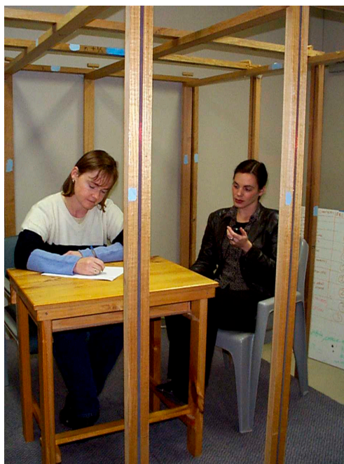
Figure 2. The ELF exposure system consisting of orthogonal square Helmholtz coils with spit windings—this allows current to flow both during sham (cancelling mode) and field (augmenting mode) to avoid audible cues due to the 50 Hz “hum”. The two sets of coils are 90° out-of-phase, giving rise to circularly-polarized fields, similar to those near power transmission lines. All items within the coils are made from non-ferrous materials. The central region with 0.8 m radius has a field uniformity within 2%.
