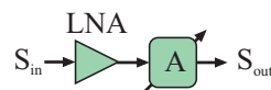
Figure 5. An automatic gain control (AGC) in the microwave domain can be formed by a low noise amplifier (LNA) followed by a variable attenuator.
