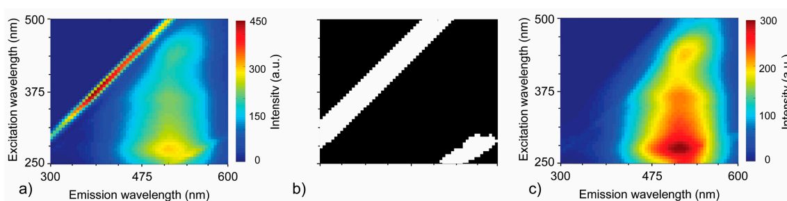
Figure 1. Results of data pre-processing: (a) raw EEM map; (b) binary mask with Rayleigh peaks marked on white; (c) final, processed data.
