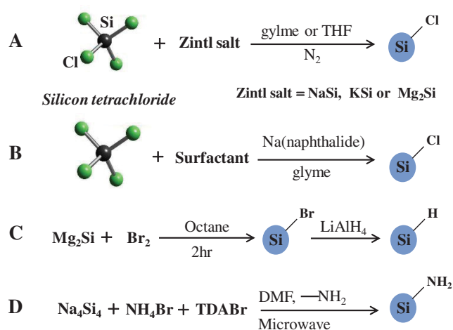
Figure 2. Schematic illustrations of heterogeneous solution-based reduction methods for preparing free-standing silicon QDs.
