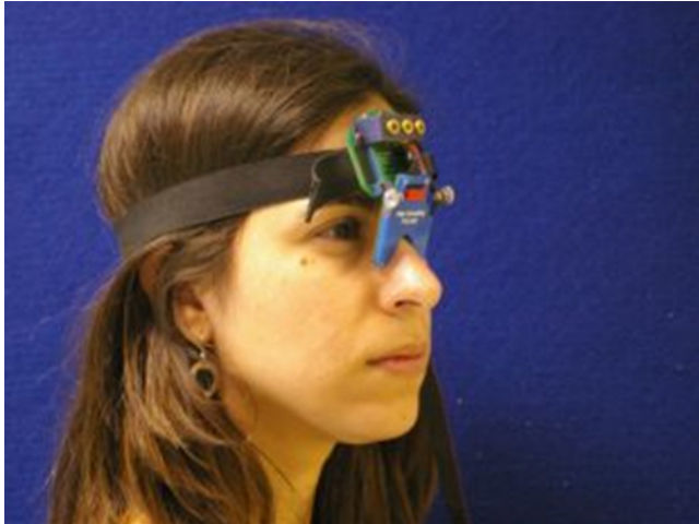
Figure 1. The Saccadometer. Head mounted saccadometer attached to an elastic band and resting on the bridge of the nose. Four miniature lasers project visual targets on to a matte surface, and the participant's eye movements are measured by differential infrared reflectance transducers on the nasal side of each eye. As the laser targets move with the head, head restraints are not required. Please click here to view a larger version of this figure.
