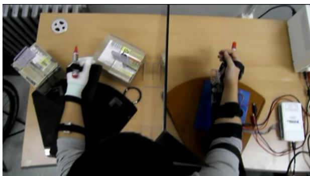
Figure 17. A Pen Marking Task in 6 Healthy Subjects using Prototype of Mirror Robot System. Conducting a pen marking task 10 times consecutively took on average 106 sec per subject.
