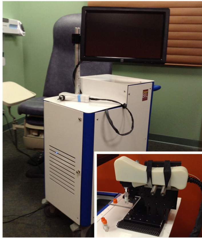
Fig. 1. Handheld optical imaging system utilizing OCT. System is designed to be portable and can be easily transported to and from clinical sites. Handheld probe utilizes interchangeable tips to allow for both a wide field-of-view during benchtop imaging as well as compatibility with speculum tips used during human subject imaging. Inset: Handheld probe in a mounted configuration used to measure phantom samples or aspirated ex vivo middle ear effusions.
