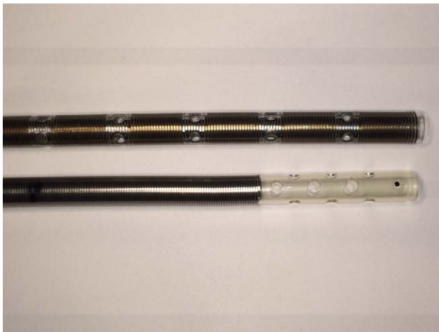
Figure 1. The different tip designs of the multistage 25 Fr/38 cm (upper cannula) and the conventional mesh 23 Fr/25 cm cannulas. The latter design drains blood through a mesh of holes at the most distal 38 mm (1½"). The multistage cannula has side holes in five segments along the most distal 102 mm (4").
