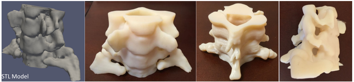
Figure 2. STL model of a spine created from a patient's non-contrast CT cervical spine examination and printed using an MRI-visible material with a high-resolution material jetting 3D printer.
