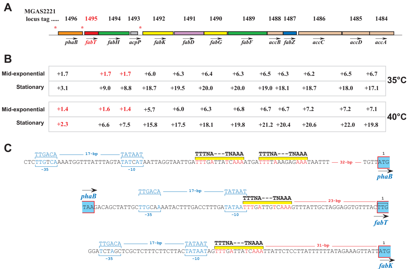
FIG 4 Regulation of fab genes by FabT. (A) The Fab cluster of GAS, showing the locations of three putative FabT-binding DNA sequences (asterisks) located in front of phaB , fabT , and fabK . fabT is depicted in red. (B) Fold expression of each gene at both temperatures and phases of growth. The values in red indicate either that the differential fold expression was below the allotted 1.5 or that the P value was excluded after applying the Bonferroni correction. (C) Figure representing the regulatory regions of phaB , fabT , and fabK , with putative promoter sequences and FabT-binding DNA sequences indicated. Nucleotide residues matching the promoter sequence and FabT site are indicated in blue and red, respectively.
