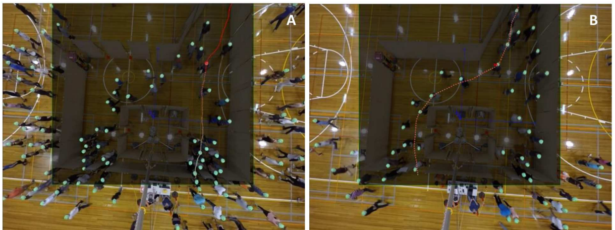
Fig 3. Raw footage of the trials is analyzed using specialty software calibrated for the specific environmental conditions in the field. Individuals are recognized and tracked by the software based on the color of the beanies they wore during the experiments. Trajectory, body movement and head orientation of each participant are inspected as external indicators to identify their likeliest decision moments. Decision moments are extracted as the moments after which participants showed most certainty and consistency in their movements. (A) A subject who chose exit 2, at their identified decision moment. (B) A subject who chose exit 3, at their identified decision moment.
