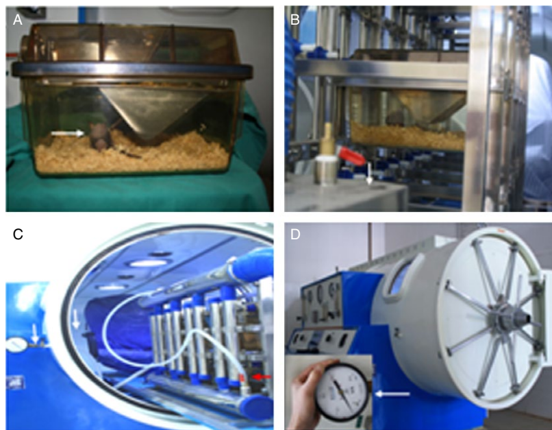
Figure 1. Hyperbaric oxygen—individual-ventilated cage (HBO-IVC) system. (A) A tumor-bearing mouse (arrow) inside the IVC; (B) fully enclosed transport channel and the air filter apparatus (arrow) connecting the feeding room to the hyperbaric oxygen therapy (HBOT) room; (C) standby HBO-IVC with plastic hose connecting the exhaust manifold (red arrow) and the pressure valve (white arrow) on the window; (D) working HBO-IVC with manometer monitoring the pressure inside IVC. The mice were divided into the four groups randomly, and each group had five mice, as shown in the Material and Methods section.
