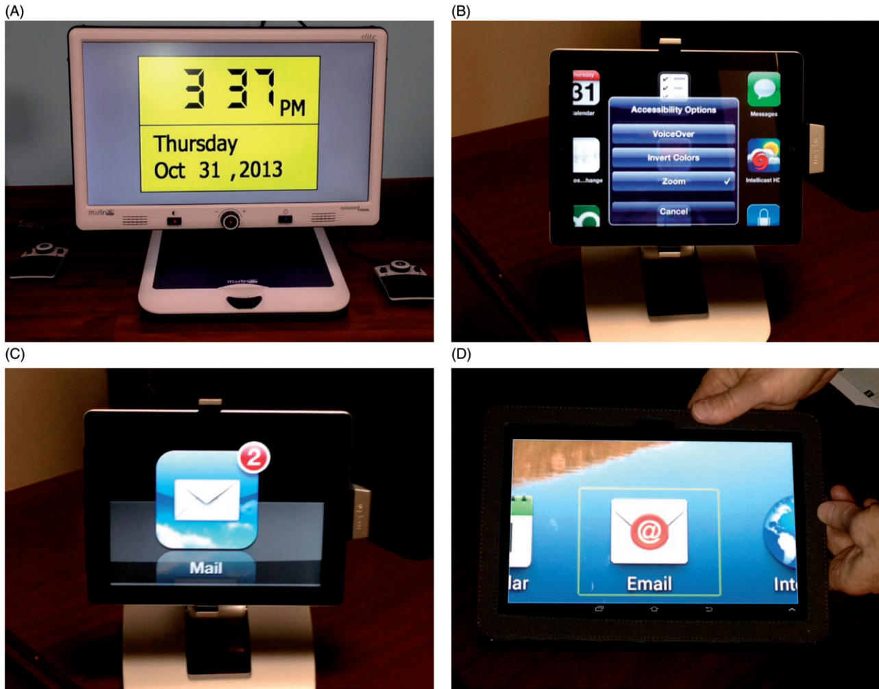
FIGURE 1 CCTVs and tablets. (A) Desktop CCTV; (B) iPad tablet with accessibility menu; (C) iPad tablet with zoom magnification activated; (D) Android™ tablet with zoom magnification activated.
