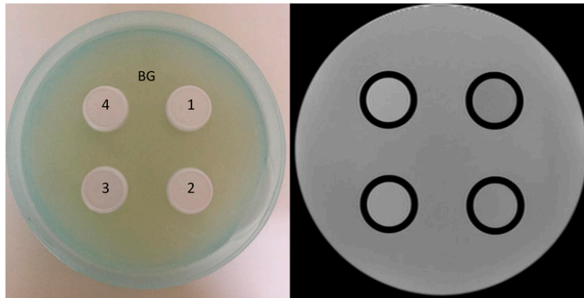
Figure 1. The photograph (left) and T_2 weighted image (right) of diffusion-weighted imaging phantom. The hemispherical plastic bottle was filled with 1.4 w/v% agar gel. Four plastic bottles were filled with 1.4 w/v% agar gel contained several concentrations of granulated sugar. The concentrations of granulated sugar of compartments 1, 2, 3 and 4 corresponded to 7.1, 14.2, 28.5 and 42.8 w/v %, respectively. BG, background.
